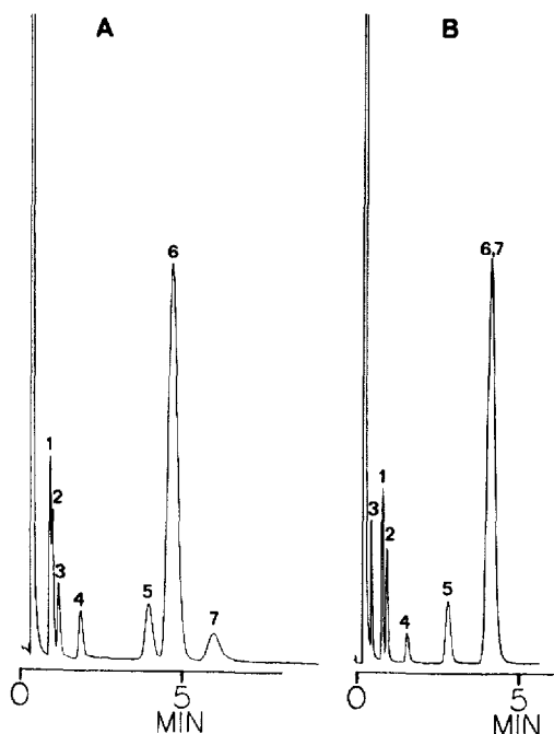
Fig. 3. Separation of a polar test mixture on matched columns of (A) QBA BuS and (B) QBA FBU S. Column 3.5 m \times 2 mm I.D. with 6.0% (w/w) salt on Chromosorb W-AW (40–60 mesh) at 131°C with a nitrogen carrier gas flow-rate of 11.0 ml/min. Peak identification: 1 = n -butylbenzene; 2 = dihexyl ether; 3 = 2-methyl-2-pentanol; 4 = 1-nitropentane; 5 = benzonitrile; 6 = naphthalene; 7 = benzodioxane.
